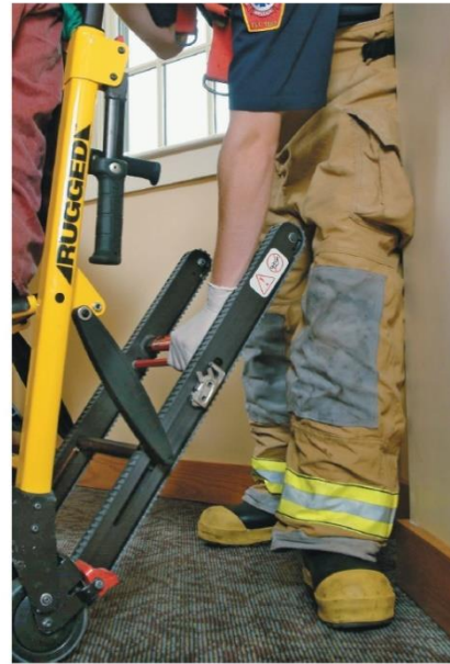
FIGURE 3-6 (A) A modern stair chair has wheels to roll the patient along a floor or level ground. (B) It also has a track that can be lowered that (C and D) allows EMTs to gently slide the patient down a staircase.
